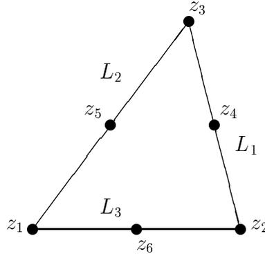
Figure 3.2: Quadratic Lagrange triangle with edges  $L_1$ ,  $L_2$ ,  $L_3$ , vertices  $z_1$ ,  $z_2$ ,  $z_3$ , and  $z_4$ ,  $z_5$  and  $z_6$  denoting the midpoints of  $L_1$ ,  $L_2$  and  $L_3$ , respectively.
