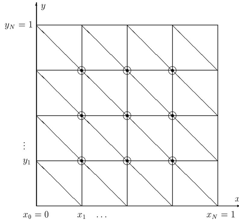
Figure 2.5: Triangulation of  $\bar{\Omega} = [0, 1] \times [0, 1]$ .
