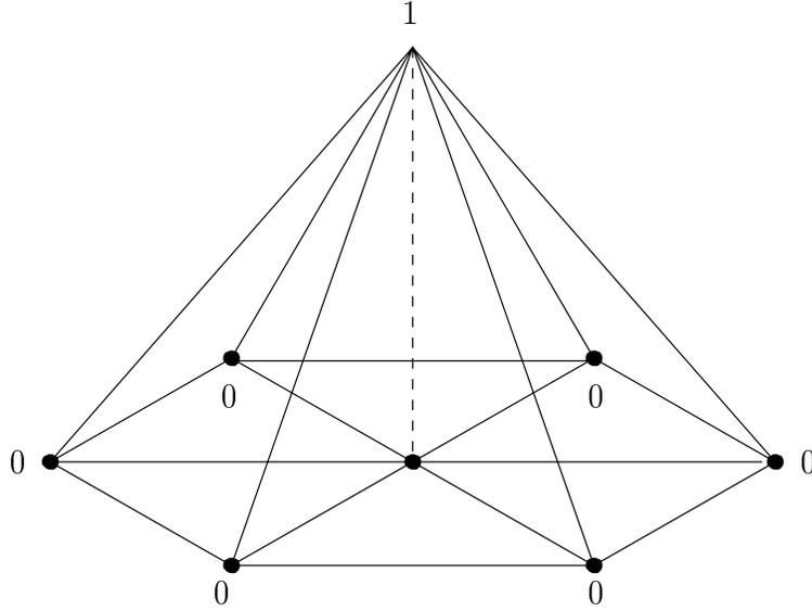
Figure 2.4: A typical finite element basis function  $\phi$ .
