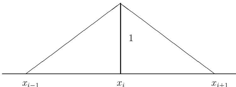
Figure 2.2: The piecewise linear finite element basis function  $\phi_i(x)$ .
