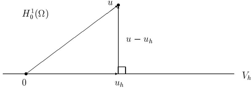
Figure 2.9: The error  $u - u_h$  is orthogonal to  $V_h$ .
